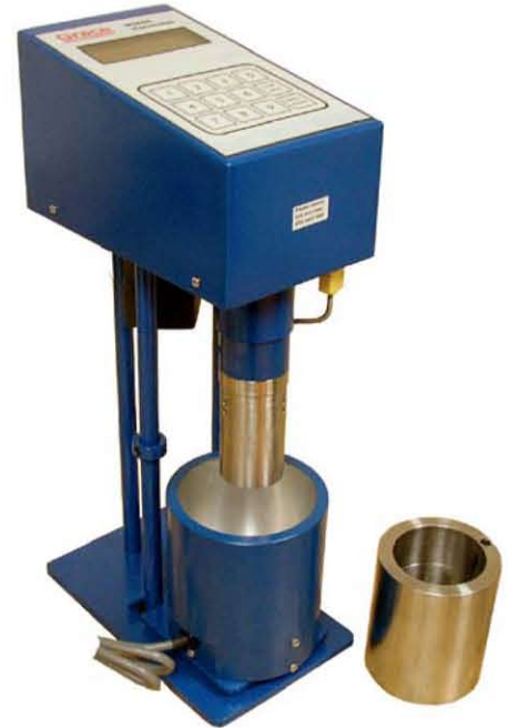
M3600 Acid Viscometer with bob
